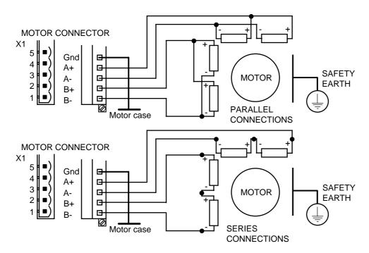
Figure 3-6. 8 Lead Motor Connection Options
